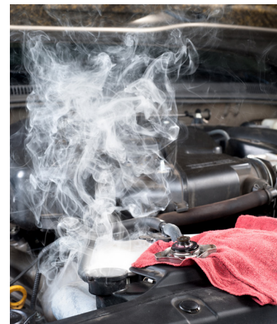
Overheated engine caused by drive belt failure.
