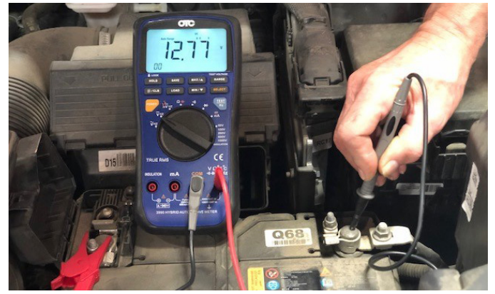
Measure the Battery State of Charge with the Ignition and all accessories off.
