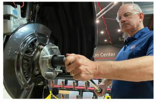
An Impact Wrench should **never** be used to tighten the Drive Axle Nut. The Impact Wrench is too imprecise and cannot accurately control the amount of torque applied. This will result in an under or over-tightened Drive Axle Nut. The vibration, "hammering," and shock from an Impact Wrench can also damage the Axle Nut, Drive Axle, and Hub Bearing.
