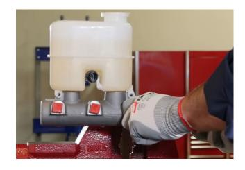
Note: Always bench bleed the master cylinder prior to installation.
