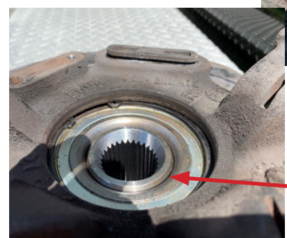
This Hub is fully seated after being pressed into the Bearing properly.
