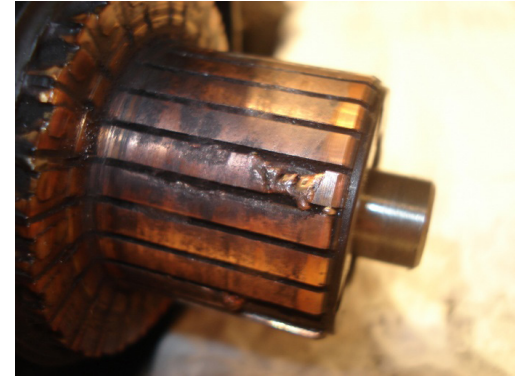
Burnt Starter Commutator from Over-cranking of the Starter
