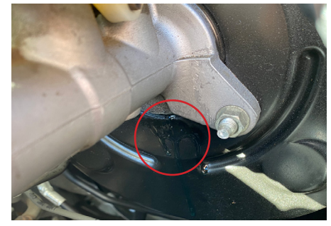
Fluid Leaking From Master Cylinder
