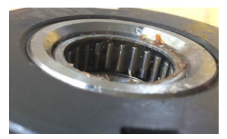
Properly Greased Needle Bearing
