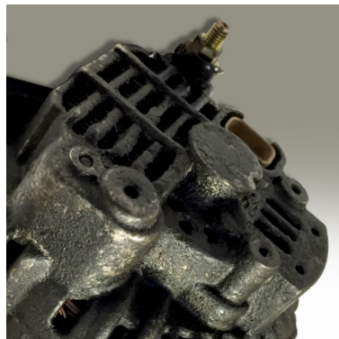
Close up view of an oil-soaked alternator.
