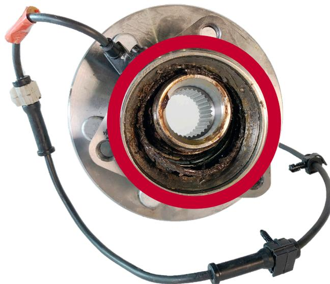
*Damaged wheel bearings may break entirely and possibly lead to serious accidents if not replaced.*
